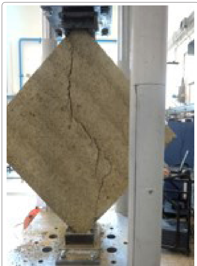
Figure 5: Failure of an URE specimen subjected to DCT.
