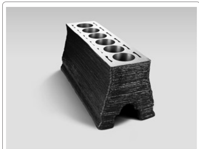
Figure 7: An example of a WAAM component [44].
