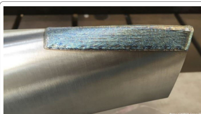
Figure 8: WAAM used to repair metal components [Image credit: CHIRON Group][47].
