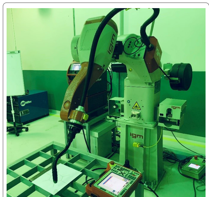
Figure 4: Robotic arm using Gas Metal Arc Welding (Robotic GMAW).
