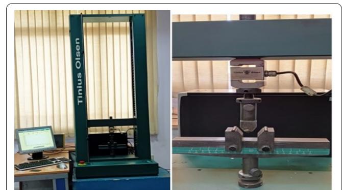
Figure 4: Tinius Olsen 10 kN (3-point bend test).
