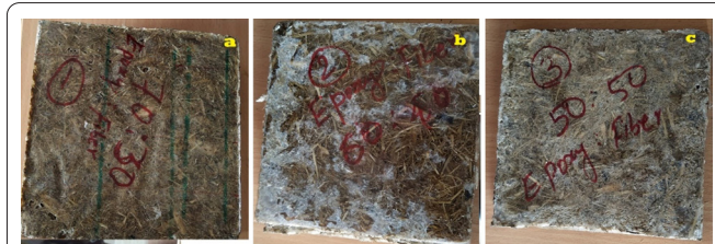
Figure 4: Fabricated Z. oenoplia - Epoxy Composite (a) Specimen 1, (b) Specimen 2, and (c) Specimen 3.
