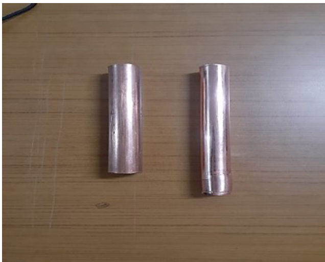
Figure 2: Original copper tube and ATB processed pass 1.
