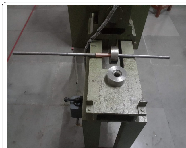
Figure 1: Experimental set up showing copper tube and Laxmi make die.
