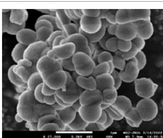
Figure 2: SEM micrograph of Se nanoparticles.
