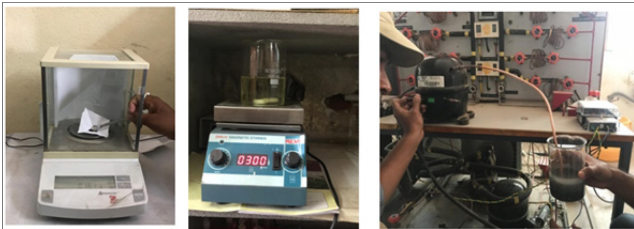
Figure 2: Adding of nanoparticles to mineral oil and injecting it to compressor.
