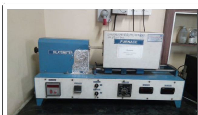
Figure 2: Dilatometer for measuring linear CTE.
