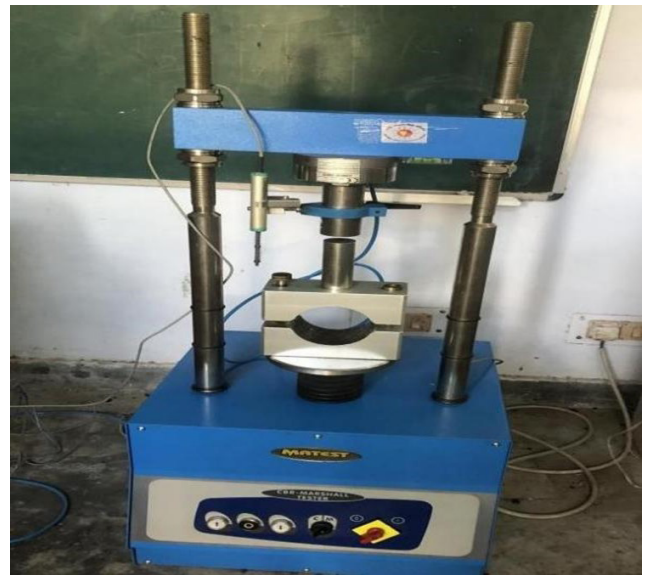
Figure 3: Marshall stability test apparatus.
