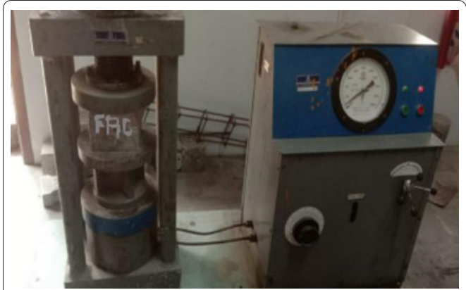
Figure 1: Compressive strength test setup.
