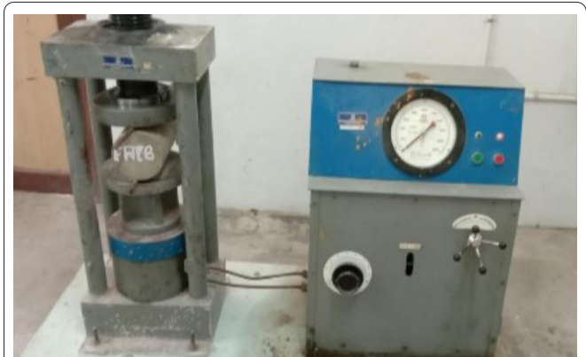
Figure 2: Split tensile test setup.
