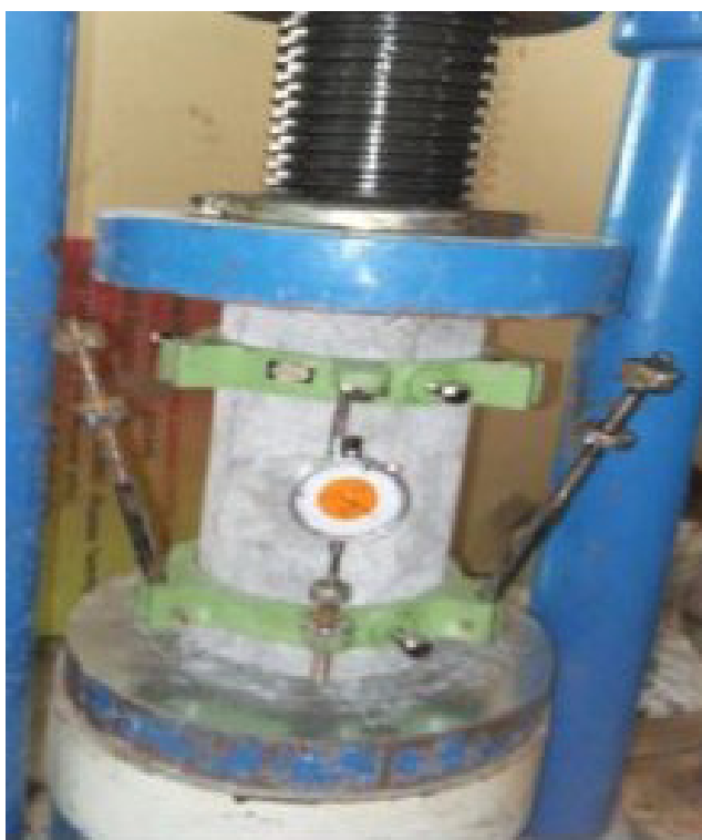
Figure 4: Modulus of elasticity test setup.
