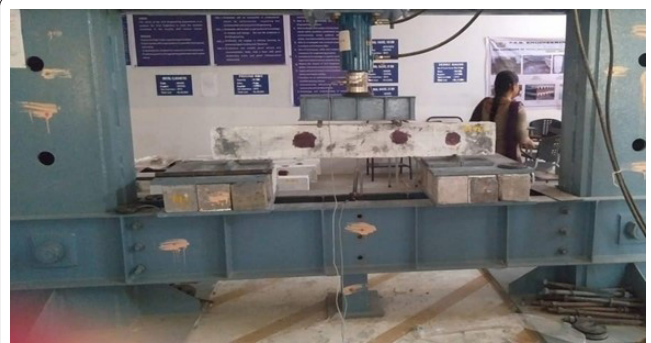
Figure 5: Flexural strength test setup.
