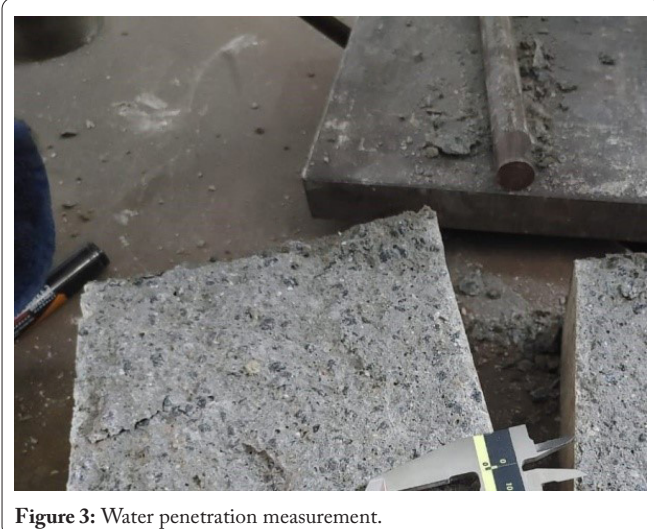
Figure 3: Water penetration measurement.
