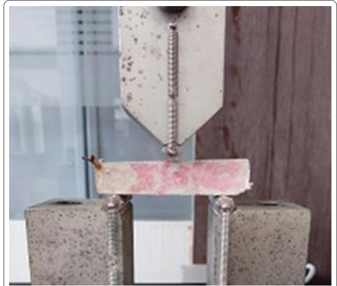
Figure 3: Flexural test of cement coir composite.
