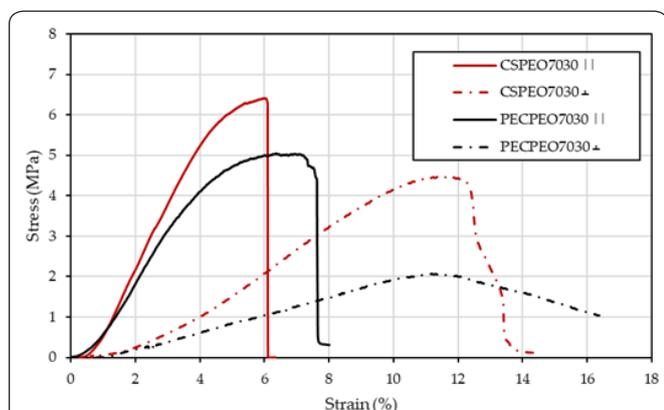
**Figure 4:** Comparison of mechanical response in dried state for aligned CS/PEO and PEC/PEO nanofibers (70/30 ratio). Tensile tests of the samples on the parallel direction (||) and the transverse (⊥) direction of nanofibers.
