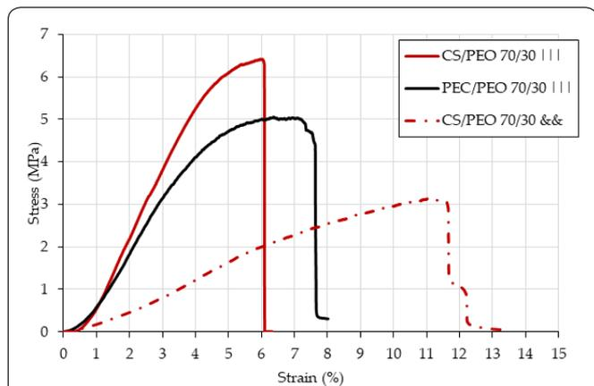
**Figure 3:** Comparison of mechanical behavior, under traction tests, of as-spun randomly collected (&&&) and unidirectional oriented (|||) PEC and CS nanofiber mats. PEC NH<sub>2</sub>/COOH = 2.35, composition polymer/PEO = 70/30. Solvent FA/W 1/1 v/v.
