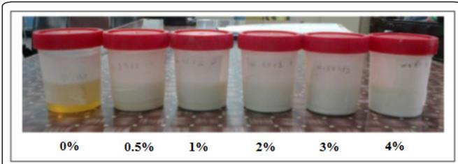
Figure 3: Samples of PAVc/TiO<sub>2</sub> nanoparticles solutions.
