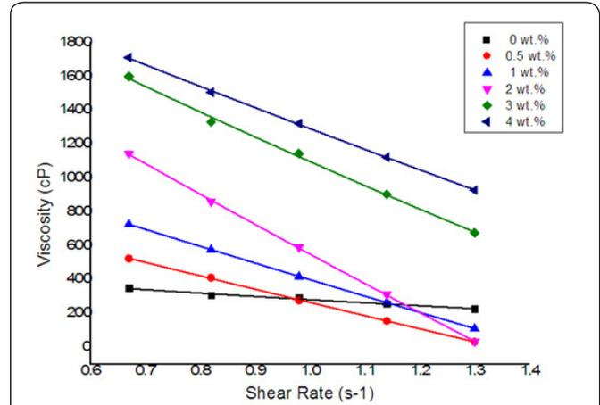
Figure 5: Viscosity behavior of PVAc/TiO<sub>2</sub> with different ratios of TiO<sub>2</sub> nanoparticles.
