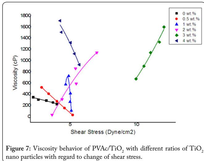
Figure 7: Viscosity behavior of PVAc/TiO<sub>2</sub> with different ratios of TiO<sub>2</sub> nano particles with regard to change of shear stress.
