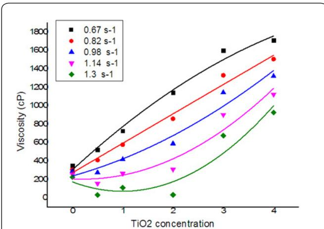
Figure 4: Viscosity behavior of PVAc/TiO<sub>2</sub> with different ratios of TiO<sub>2</sub> nano particles with regard to change of shear rate.
