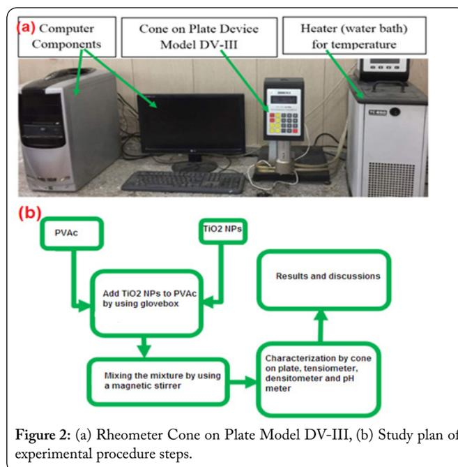
Figure 2: (a) Rheometer Cone on Plate Model DV-III, (b) Study plan of experimental procedure steps.
