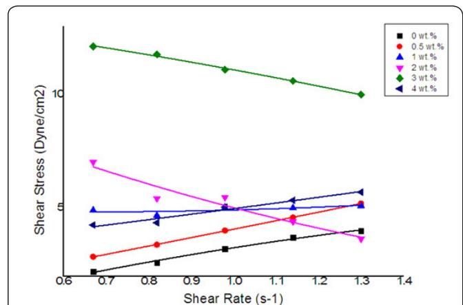
Figure 6: Shear stress - shear rate behavior of PVAc/TiO<sub>2</sub> with different ratios of TiO<sub>2</sub> nano particles.
