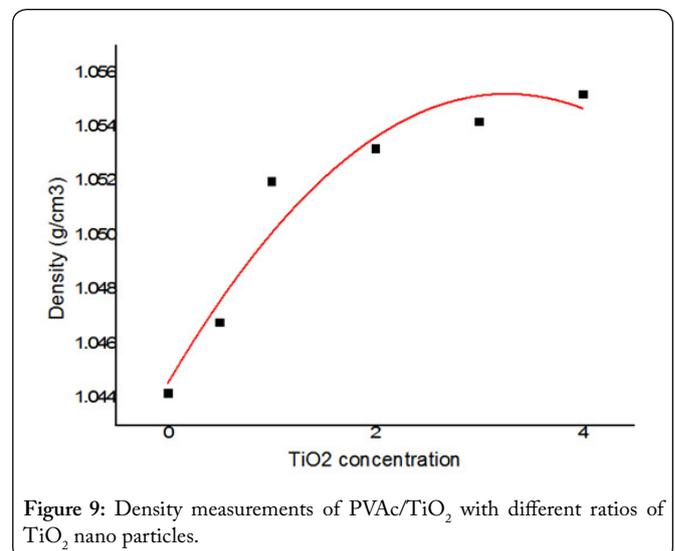
Figure 9: Density measurements of PVAc/TiO<sub>2</sub> with different ratios of TiO<sub>2</sub> nano particles.
