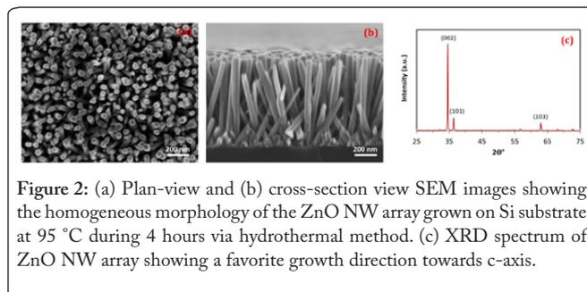
Figure 2: (a) Plan-view and (b) cross-section view SEM images showing the homogeneous morphology of the  $\text{ZnO}$  NW array grown on Si substrate at  $95$  °C during 4 hours via hydrothermal method. (c) XRD spectrum of  $\text{ZnO}$  NW array showing a favorite growth direction towards c-axis.
