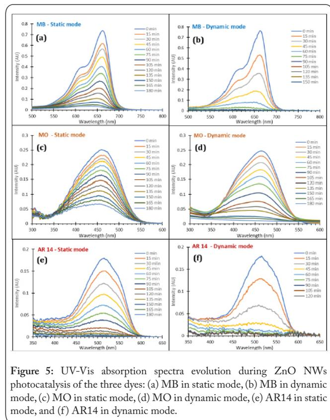
Figure 5: UV-Vis absorption spectra evolution during ZnO NWs photocatalysis of the three dyes: (a) MB in static mode, (b) MB in dynamic mode, (c) MO in static mode, (d) MO in dynamic mode, (e) AR14 in static mode, and (f) AR14 in dynamic mode.
