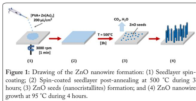
Figure 1: Drawing of the  $\text{ZnO}$  nanowire formation: (1) Seedlayer spin-coating; (2) Spin-coated seedlayer post-annealing at  $500$  °C during 3 hours; (3)  $\text{ZnO}$  seeds (nanocrystallites) formation; and (4)  $\text{ZnO}$  nanowire growth at  $95$  °C during 4 hours.
