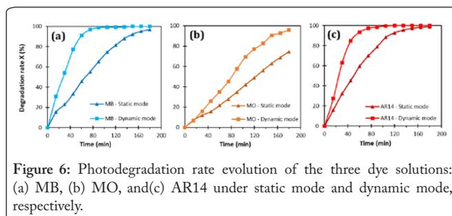
Figure 6: Photodegradation rate evolution of the three dye solutions: (a) MB, (b) MO, and (c) AR14 under static mode and dynamic mode, respectively.
