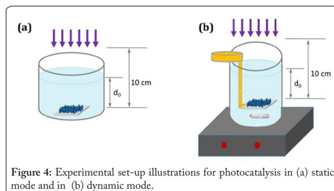
Figure 4: Experimental set-up illustrations for photocatalysis in (a) static mode and in (b) dynamic mode.
