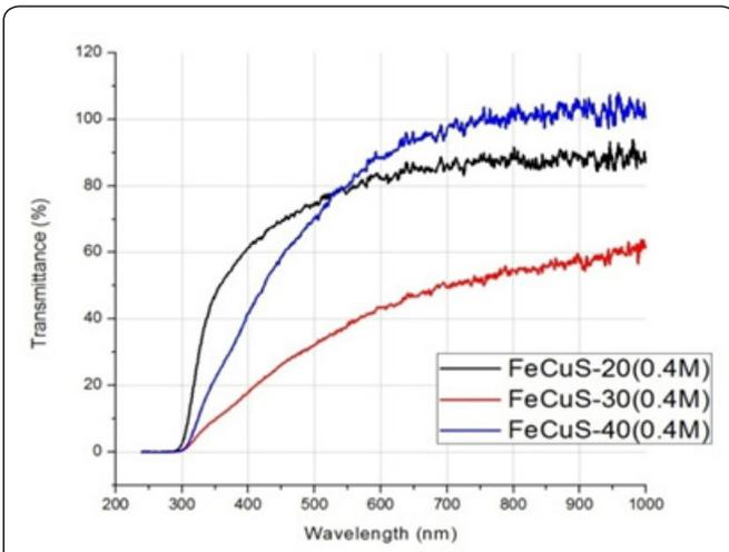
Figure 2: Graph of transmittance against wavelength of the grown thin films.
