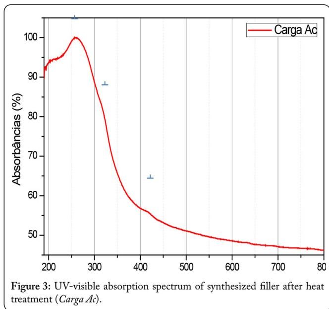
Figure 3: UV-visible absorption spectrum of synthesized filler after heat treatment (Carga Ac).
