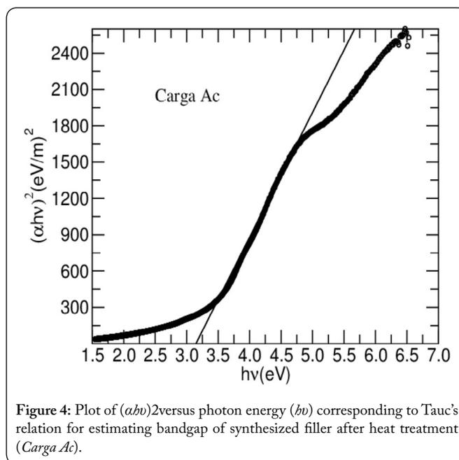
Figure 4: Plot of  $(\alpha h\nu)^2$  versus photon energy ( $h\nu$ ) corresponding to Tauc's relation for estimating bandgap of synthesized filler after heat treatment (Carga Ac).
