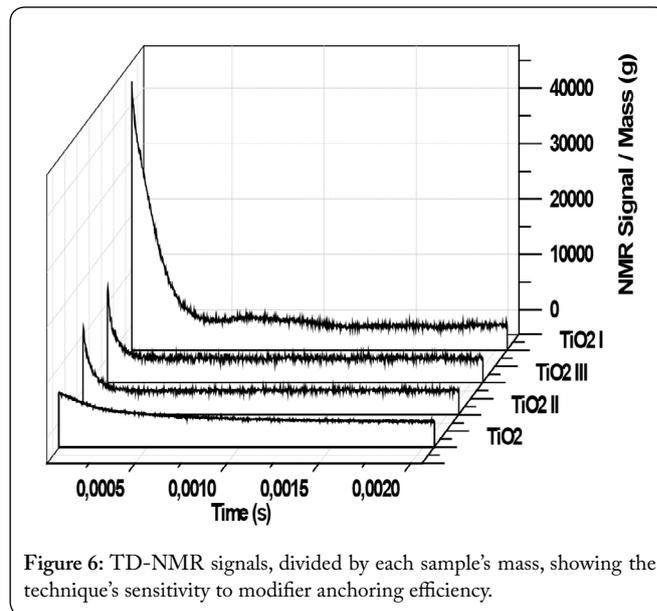
Figure 6: TD-NMR signals, divided by each sample's mass, showing the technique's sensitivity to modifier anchoring efficiency.
