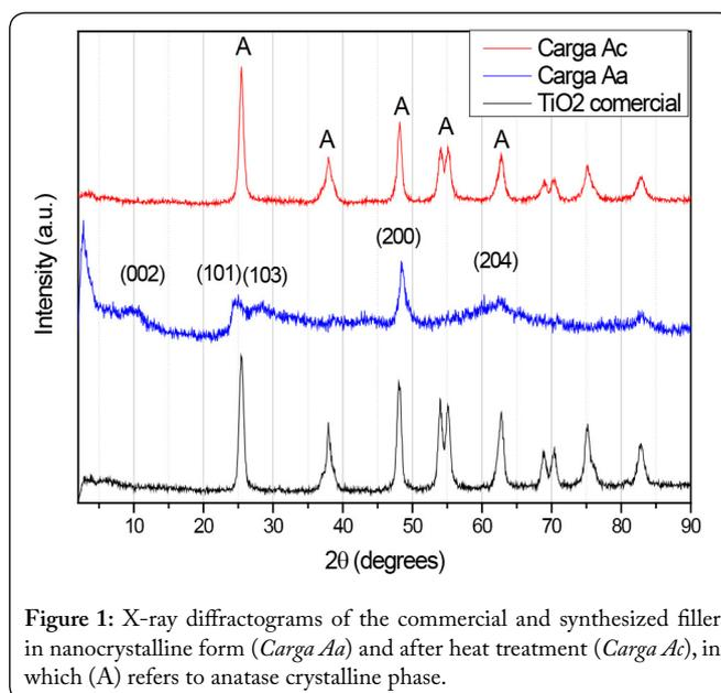
**Figure 1:** X-ray diffractograms of the commercial and synthesized filler in nanocrystalline form (*Carga Aa*) and after heat treatment (*Carga Ac*), in which (A) refers to anatase crystalline phase.
