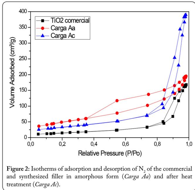
Figure 2: Isotherms of adsorption and desorption of N<sub>2</sub> of the commercial and synthesized filler in amorphous form (Carga Aa) and after heat treatment (Carga Ac).
