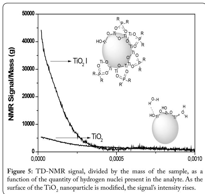
Figure 5: TD-NMR signal, divided by the mass of the sample, as a function of the quantity of hydrogen nuclei present in the analyte. As the surface of the  $\text{TiO}_2$  nanoparticle is modified, the signal's intensity rises.
