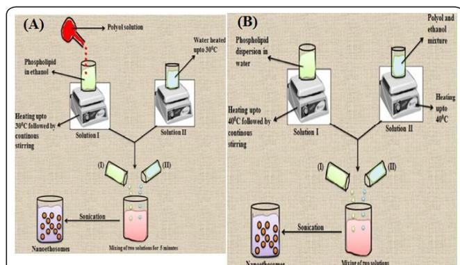
Figure 3: Preparation of nanoethosomes by cold and hot technique. (A) Cold technique involves mixing of two solutions at a low temperature of 30 °C, and (B) hot technique involves mixing of two solutions at a high temperature of 40 °C.
