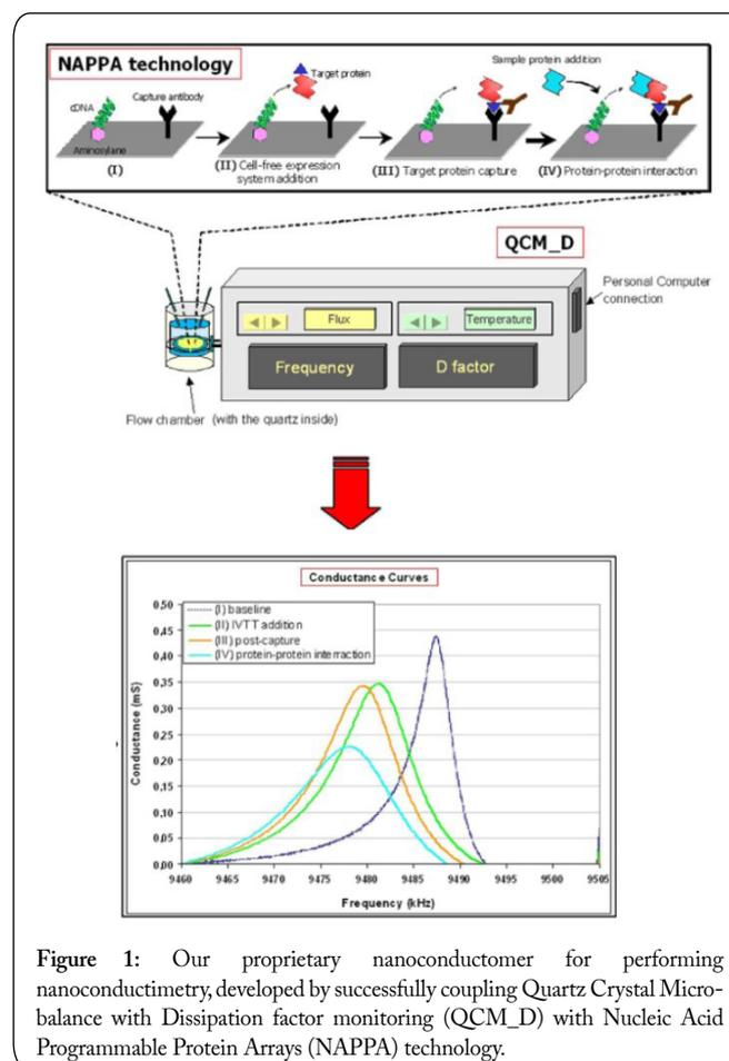
Figure 1: Our proprietary nanoconductometer for performing nanoconductimetry, developed by successfully coupling Quartz Crystal Microbalance with Dissipation factor monitoring (QCM\_D) with Nucleic Acid Programmable Protein Arrays (NAPPa) technology.
