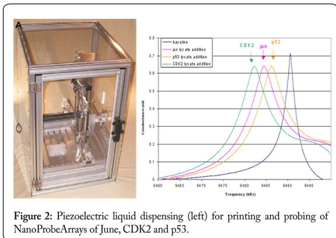
Figure 2: Piezoelectric liquid dispensing (left) for printing and probing of NanoProbeArrays of June, CDK2 and p53.
