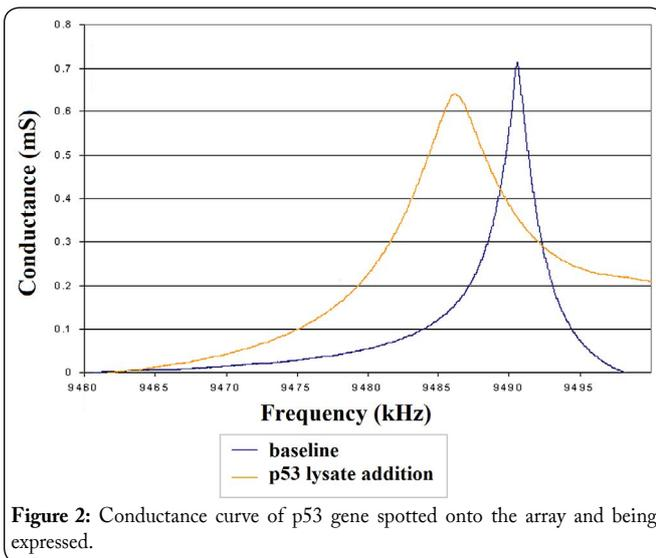
Figure 2: Conductance curve of p53 gene spotted onto the array and being expressed.
