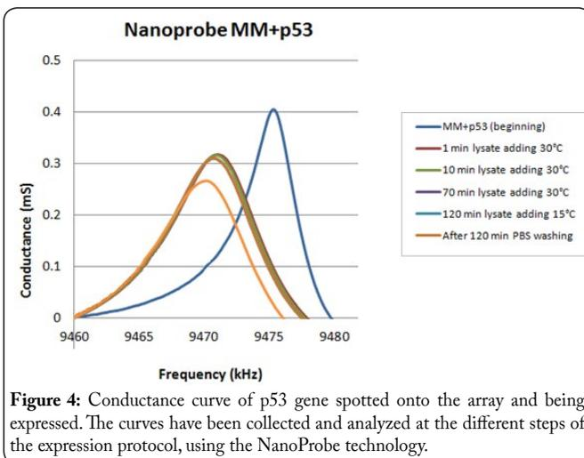
Figure 4: Conductance curve of p53 gene spotted onto the array and being expressed. The curves have been collected and analyzed at the different steps of the expression protocol, using the NanoProbe technology.
